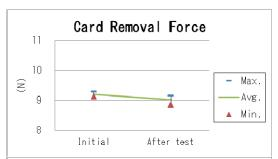
Card Insertion Force: The load for cum-lock Card Removal Force: The load for cum-unlock
